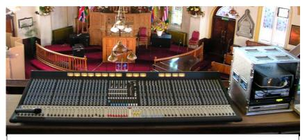
An Allen & Heath ML4000 48 Channel Mixing Console is the nerve centre for the audio system. It offers VCA and Group Busses, LCR Control, Matrix Outputs, 12 Monitor Auxiliaries, PC Snapshot Memories and pristine sound quality.
