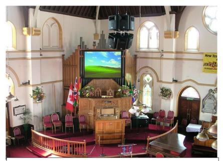
The main church showing six flown Electrovoice SX300 speakers with two 2 x 18" subwoofers below – powered and controlled by EV and DBX amplification and processing.
